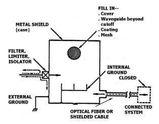
Figure 39. Box-level hardening techniques
