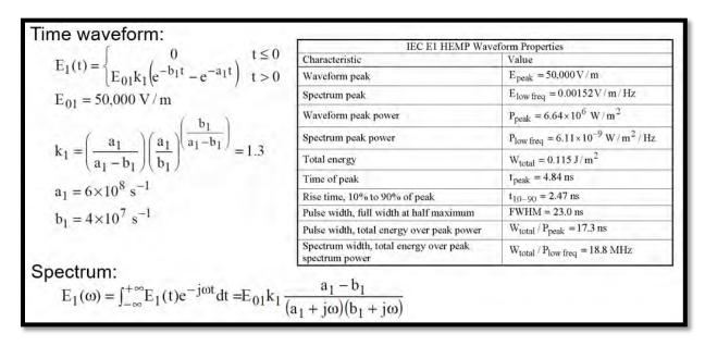
Figure 2. IEC Standard E1 Waveform (ref. IEC 61000-2-9)
