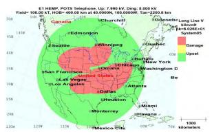
Figure 45. Devastating POTS telephone damage with 0 dB protection
