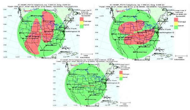
Figure 25. Protective effects on a Plain Old Telephone Service Line with 30 dB shielding
