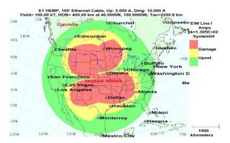
Figure 41. Potential upset/damage of equipment connected to 100' Ethernet cable with 0 dB protection
