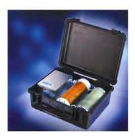
Figure 17. DIEHL Munitions damped sine IEMI generator
