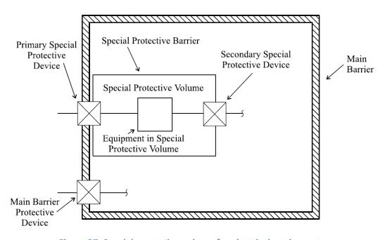
Figure 37. Special protective volume for electrical equipment
