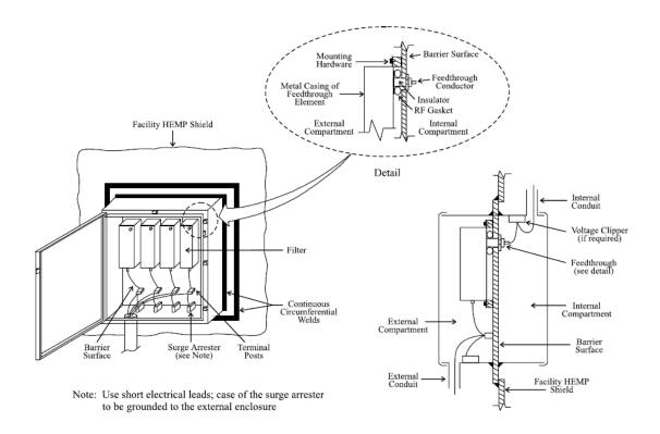
Figure 27. Typical cable POE protection design
