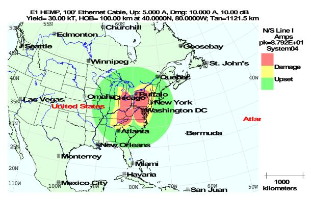
Figure 10. Potential disruption for 100' Ethernet-connected equipment from 30 kT HEMP
