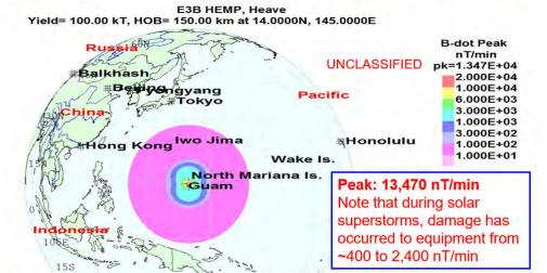
Above: A 100 kT "generic" nuclear weapon detonated at 150 km altitude above Guam could generate a powerful low frequency "heave" E3B pulse that could couple into power lines and other long conductors, such as undersea cables. This graphic shows that Guam is covered by significant, low frequency EMP for a period of up to 300 seconds after the burst (at levels up to a maximum of 13,470 nanoteslas/minute).
