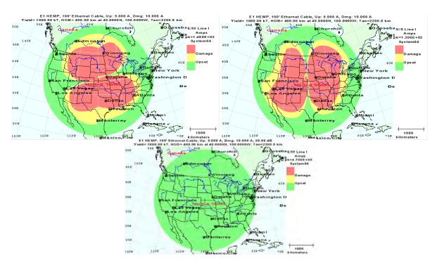
Figure 24. Protective effects on a 100' Ethernet cable with recommended 30 dB shielding
