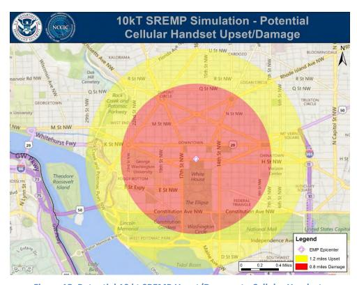
Figure 15. Potential 10 kt SREMP Upset/Damage to Cellular Handsets
