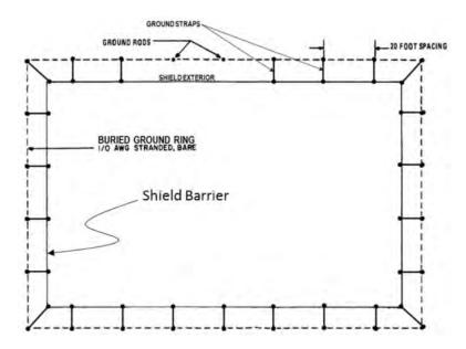
Figure 34. Shield barrier earth electrode system
