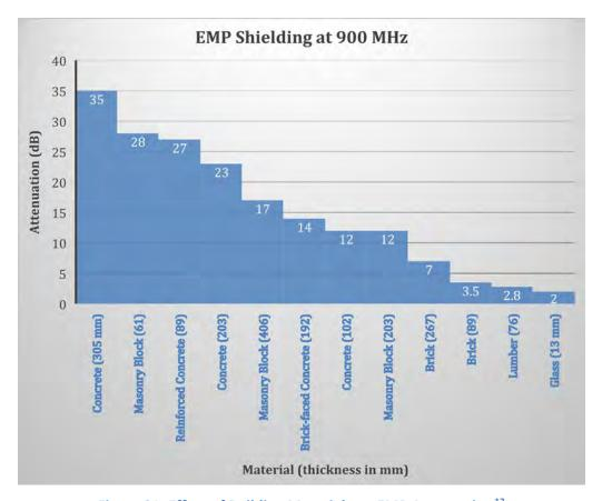
Figure 21. Effect of Building Materials on EMP Attenuation<sup>13</sup>
