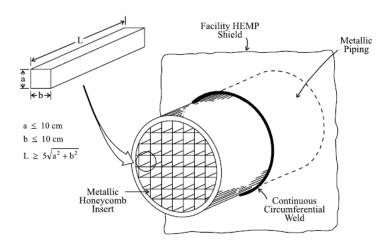
Figure 32. Typical waveguide-below-cutoff (WBC) piping POE protective design for E1 HEMP
