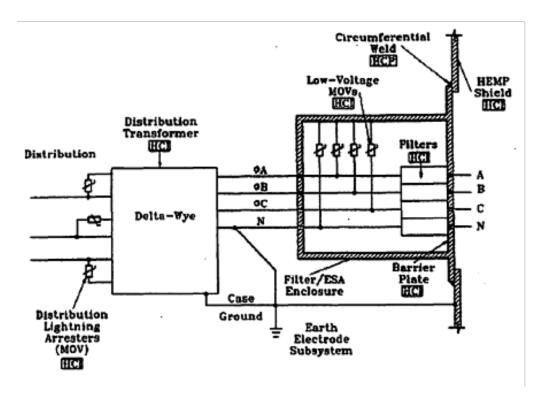
Figure 28. Commercial electric power POE protection
