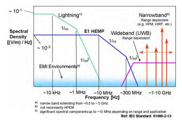
Figure 8. Frequency ranges of Lightning, HEMP, and IEMI <sup>3</sup>
