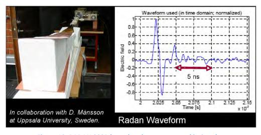
Figure 19. RADAN 303B hyperband generator used in Sweden
