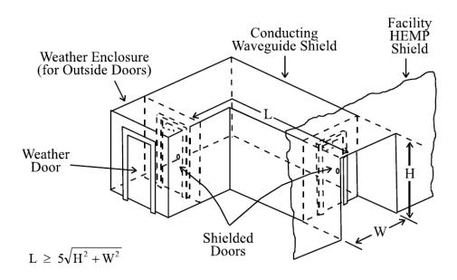
Figure 30. Entryway using two doors separated by a WBC <sup>14</sup>
