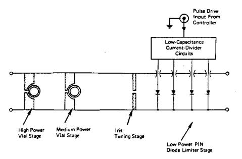
Figure 35. Example receiver protector unit diagram.
