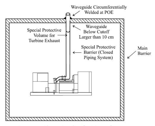
Figure 36. Special protective volume for piping POE for E1 HEMP
